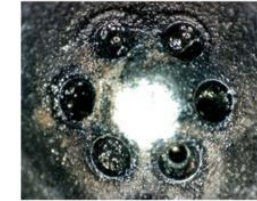
Injector nozzle before cleaning
