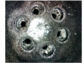
Injector nozzle after cleaning
